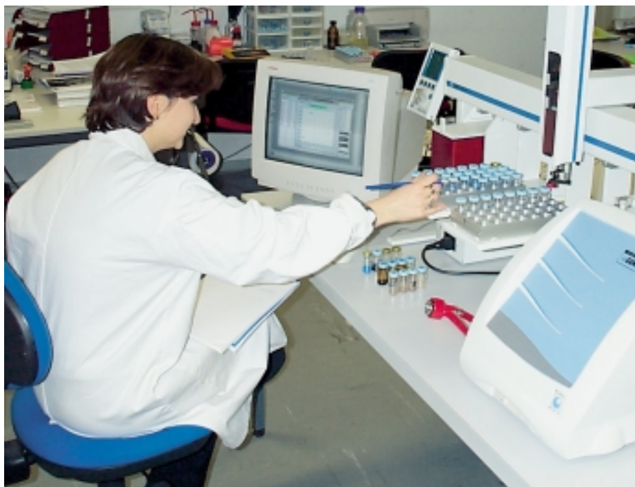
Fig. 1: \alpha Gemini system equipped with a 64-position autosampler located in QC laboratory
