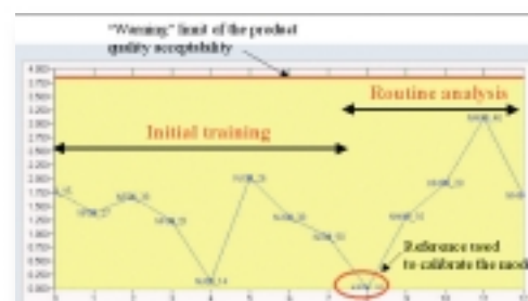
Fig. 2: Statistical Quality Control chart showing the initial training step of the quality variability followed by the analysis of unknown batches
